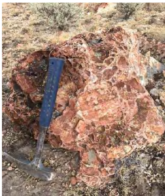
Photo 1 Strongly illitized fragments of Tr in frontal breccia Trf with incipient chalcedonization around fragments. These are more strongly illitized than most, and is easily eroded, thus few outcrops exist (most areas of illitized rock are based on mapping of float).
